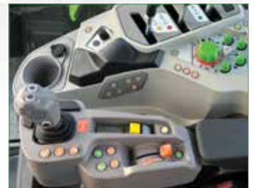
20 SPEED ELECTRONIC ARMREST CONTROLLED FULL POWERSHIFT TRANSMISSION
