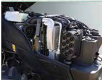
HIGH FLOW 100 L/MIN CLOSED CIRCUIT HYDRAULIC SYSTEM
