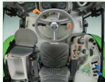
PRO-VISION CAB WITH PNEUMATIC SUSPENSION SEAT AND TRAINEE SEAT
